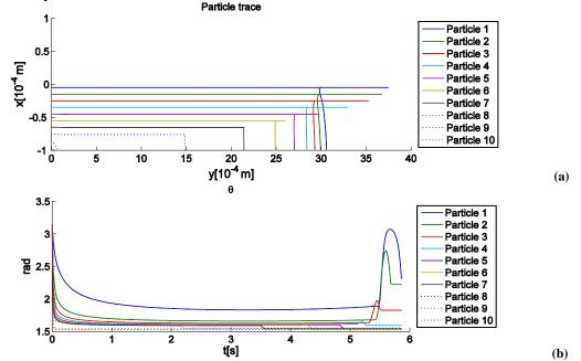
**Figure 2:** (a)*The trace left by ten oblate particles released at t=0 and evenly distributed along the negative x axis.* (b) *The angle between the normal vector of the particles and the y axis as a function of time*
